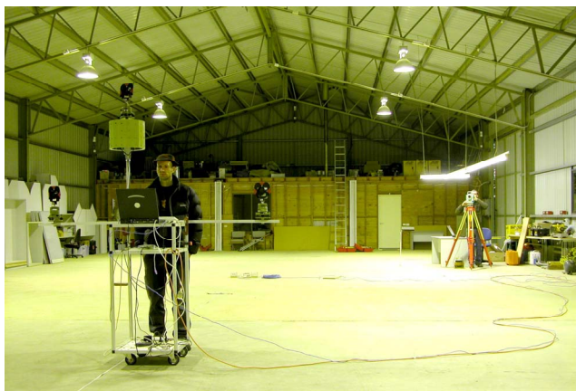
Fig. 5. Indoor test site, Locata receiver on trolley and RTS setup.
