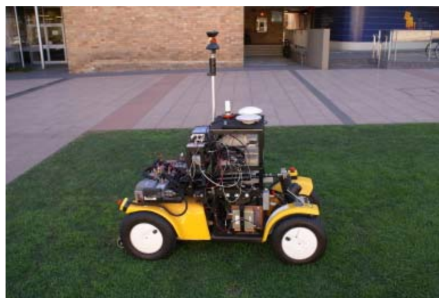
Fig. 3. Integrated GPS+INS+Locata test car on UNSW campus.
