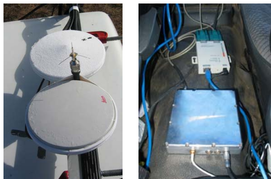
Figure 8. Locata and GPS setup: antennas mounted on truck roof (left), and Locata receiver connected to Lantronics serial-to-TCP/IP converter.
