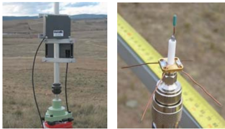
Figure 4. LocataLite LP patch antennas (left), and Locata receiver \frac{1}{4} wave antenna (right).
