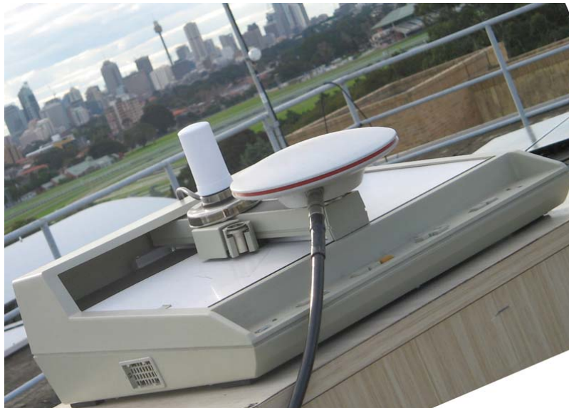
Figure 5 HP XY plotter table with Locata and Leica AT502 antennas.
