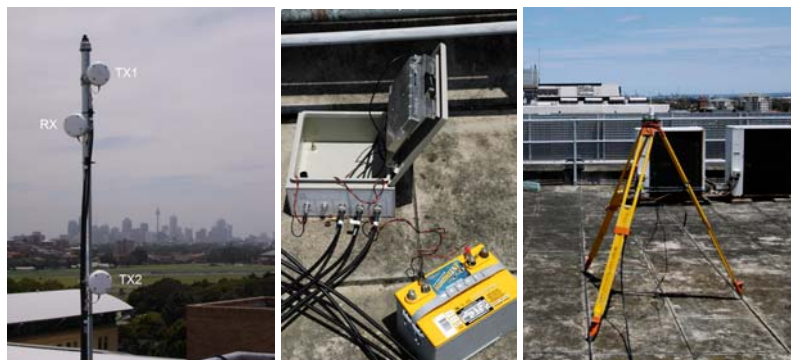
Figure 2 LocataLite (5) antenna setup (left) and weatherproof enclosure (middle). Locata receiver antenna setup (right).
