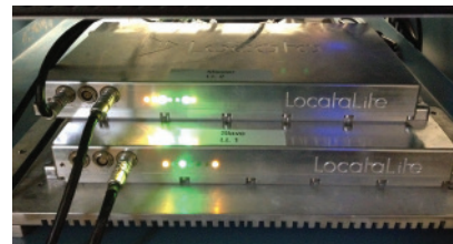
▲ FIGURE 2 LocataLites under test at USNO
