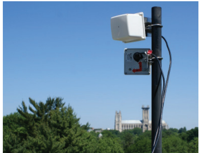
▲ FIGURE 9 LocataLite antennas on USNO Building 1. National Cathedral in background.
