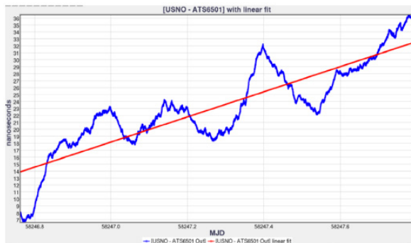
FIGURE 8. USNO versus timing receiver with linear fit.
