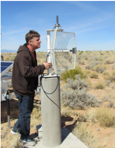
TECHNICIANS WITH THE 746 TS re-aim a LocataLite antenna for an alternative TimeLoc configuration (left), and with USNO personnel, reconfigure the Master LocataLite site for the test.
